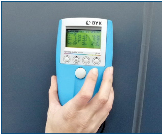
Photo 11 – Measurements of finish gloss using a color spectrophotometer.
